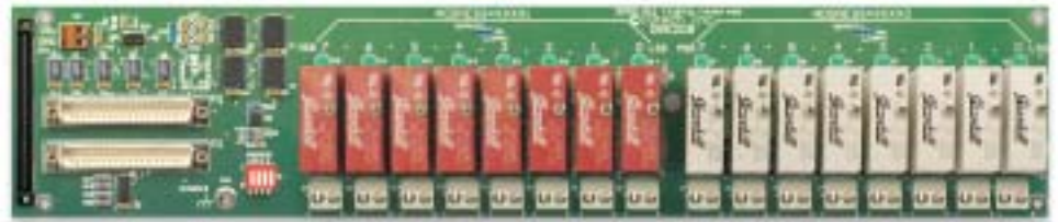
The DBK208 accepts up to 16 isolated solid-state-relay (SSR) digital I/O modules
